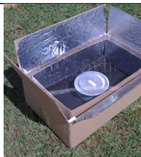
Fig. (13): A model for Solar Cooking. Made and demonstrated onsite
